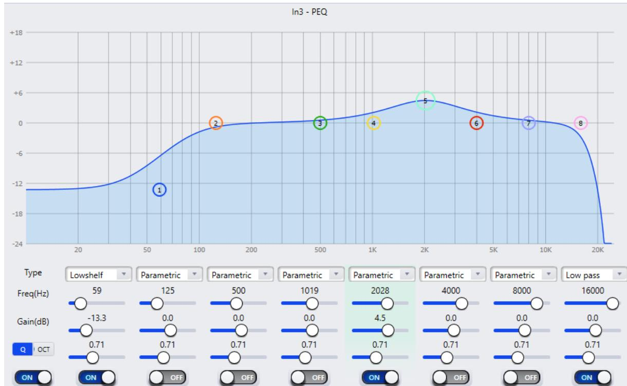
**Frequency (Hz):** Determines the center frequency of the filter.
