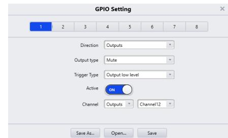
**Save As...:** Save the current GPIO configuration to a file. This can be done offline for commissioning at a later stage or saving record of configurations for a finished project.
