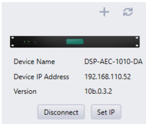
Click the **+** to manually add devices based on IP address if for example devices are located in a different broadcast domain and can't be discovered automatically.
