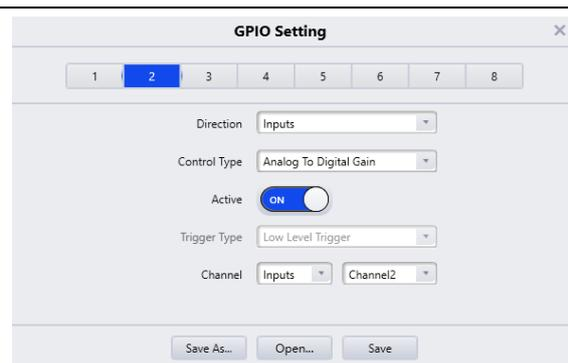
**Channel:** 8 channel buttons select the channel to be configured.
