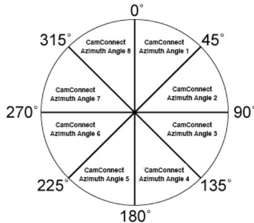
If the forbidden area is enabled on the Sennheiser Control Cockpit software, the corresponding position of CamConnect will also be affected. Example: If the forbidden area is set to 0° to 60°, the audio signal from 0° to 45° of CamConnect Array Azimuth 1 and 45° to 60° of Array Azimuth 2 will be ignored.
