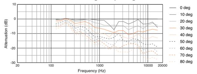
Measurements obtained in bi-amp mode using FIR filters. Graphs are from unaltered measured data.
