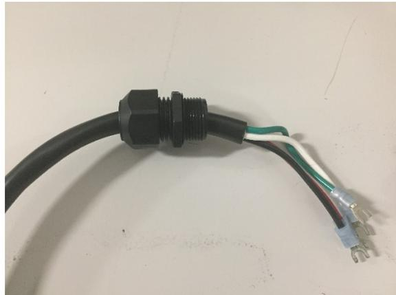
Remove washer from gland nut, add Gland Nut Cover to cable and replace washer and tighten around gland nut. Do not tighten the main gland nut yet.
