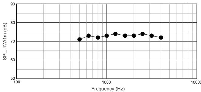
Contribution of each mid-range one-third-octave frequency band to the SPL (per EN54-24) when system is driven to Rated Maximum SPL (89 dB @ 4m; 101 dB @ 1m) using specified broadband pink-noise signal, 60W tap setting, 1m (Contribution figures: 500 Hz = 71 dB; 630 Hz = 73 dB; 800 Hz = 72 dB; 1000 Hz = 73 dB; 1250 Hz = 74 dB; 1600 Hz = 73 dB; 2000 Hz = 73 dB; 2500 Hz = 74 dB; 3150 Hz = 73 dB; 4000 Hz = 72 dB).
