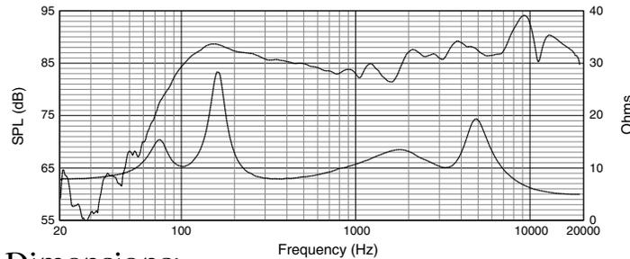
Frequency Response chart (2 $\pi$ , mounted in ceiling), 100V input on 25W tap, measured at 4 meters
