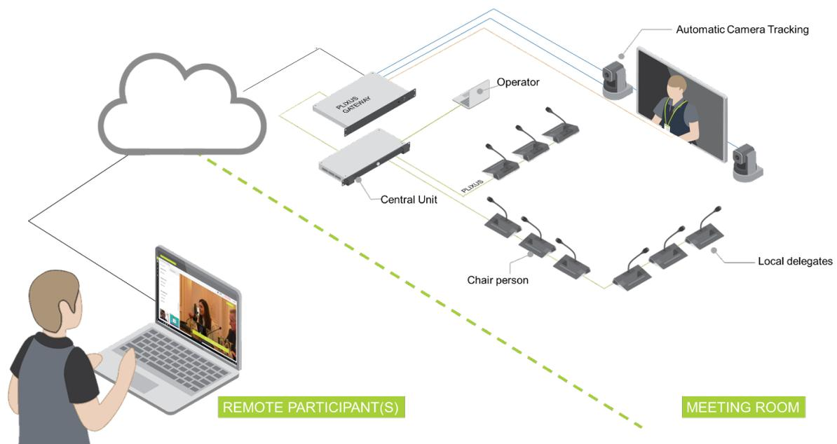
Figure 1-1 Typical Plixus Gateway setup where the gateway is connected to the Cloud, the Central Unit, the screen and the cameras
