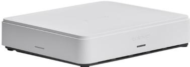
Confidea WAP G4 controls all communication to and from the Confidea FLEX G4 Wireless units. It can be used for meeting management, and comes with both analog and digital audio interfaces, as well as recording capabilities.
