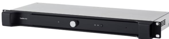
Plixus AE-R is an embedded system for meeting management that provides all the processing and signal handling required for the Plixus network. It comes with both analog and digital audio interfaces, controls the delegate units and interconnects other audio systems. A record button also allows to start and stop the audio recording of the meeting.
