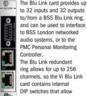
a block of 32 sequential channels from the 256 to be addressed by the card, separately selectable for inputs and outputs.
