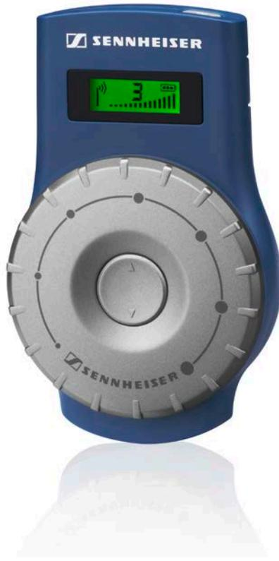
The EK 2020-D-II is a sturdy digital RF bodypack receiver. It works in the frequency range of 863 – 865 MHz and offers 6 channels in parallel in tourguide mode, 8 channels in the conference mode in combination with a stationary transmitter. Intuitive operating controls make it easy to use. The included lithium polymer battery offers 16 hours of battery life. It can either be used with headphones or induction loops for use with hearing aids.
