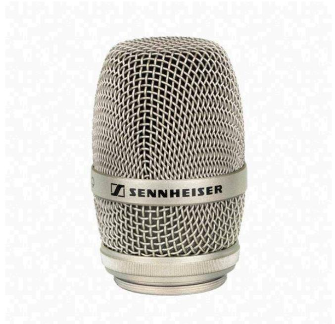
This microphone head with a true condenser capsule in large-diaphragm technology showcases Sennheiser's unrivaled experience in the fields of acoustics and stage technology. Its powerful, high-definition sound makes it one of the best microphone heads of all time. Because of its dual-membrane technology, the pick-up pattern can be switched between cardioid and super-cardioid.
