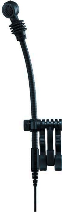
The e 608 has a newly developed clamp and gooseneck mounting, which enables the capsule to be positioned close to the signal source for high realism and high level output. Extensive damping and shock mounting isolates the capsule and signal from extraneous vibration, noise and impact.
