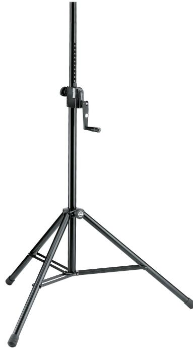
A high quality steel speaker stand with zinc die-cast clamps for professional use. Infinitely variable height adjustment with a hand crank and push button system which prevents an uncontrolled reverse motion. There is an additional locking screw for extra safety. Extension tube diameter 35 mm, suitable for speakers and lighting crossbars with an integrated M10 thread connector.
