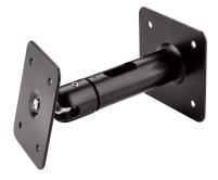
The practical wall and ceiling mount for smaller loudspeakers has been upgraded. A new feature is a cable outlet, which now provides an internal cable guide for hidden installations. Thanks to two special threaded pins and the Allen wrench / hexagon key included in the delivery, the universal joint can be positioned and set exactly. As such the load-bearing capacity increases to 10 kg. The wall distance has been reduced to 160 mm.
