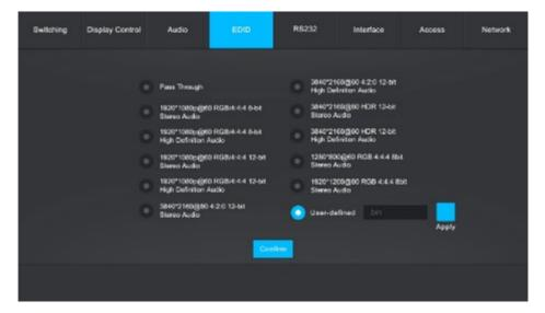
**Note:** Before select EDID in this tab, please ensure the 4-pin DIP switch on the rear panel is on the "1111" position.
