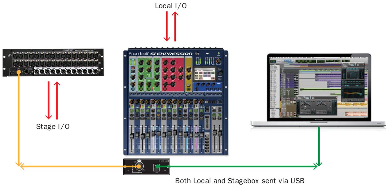
Providing the Dipswitches are set as above and the Stagebox is connected, clocked and receiving audio, channels will be sent from the Stagebox through the console and straight out to the DAW for recording. Due to the freely assignable architecture of Si Consoles, Direct out patches and input patches can be made from anywhere, to anywhere on the console for maximum flexibility.
