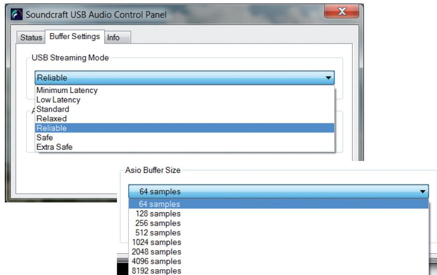
For example, by setting the streaming mode to 'Reliable' and then the buffer size to 1024 samples, the system will then be running at 1024 samples and the audio will be clean. For lower buffer sizes, the streaming mode should be set to 'Low Latency' and the buffer size to 128 samples.
