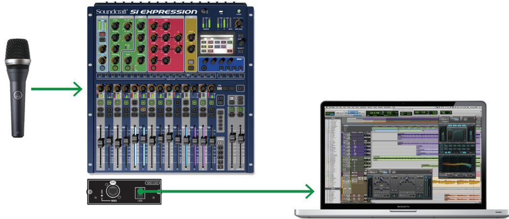
The MADI-USB Combo card also enables multi-track recording and playback. Standard mic/line input sources can be recorded through the Si series console via the card to a DAW or similar. This simple yet powerful solution is suitable for recording live gigs but is equally at home in the studio.
