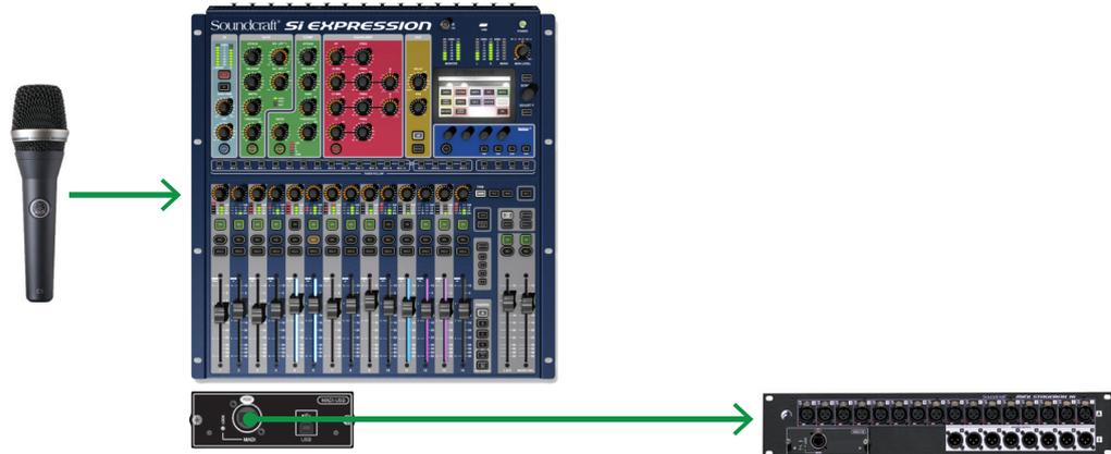
MADI is a standard protocol on all Soundcraft Stageboxes including the Compact Stagebox and Vi Stagebox. The connection to a Stagebox works exactly the same for all Soundcraft consoles and Stageboxes.
