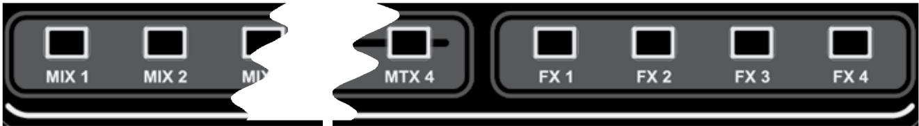
These keys place the console into 'MIX' mode allowing quick & easy mixing from Channels to Buses, Channels to FX or Buses to Matrix. Pressing any key triggers a sequence of events that re-configure the control surface and console monitoring system to the optimum layout for the desired/required function.
