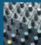
The MFXi/MPMi consoles use vertically mounted PCBs which are secured with nutted pots for extra strength, stability and easy servicing. Well-spaced controls provide easy access at those critical control moments, enhanced by clear legending which highlights linked or associated functions.
