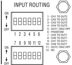
CSM 28 include a default routing of input channels 1-4 to output 1 and input channels 5-8 to output 2. The user may also take any input and have it routed to both outputs by selecting the appropriate switch. For example, if you set switch 1 to ON, it will be routed to both OUT1, and OUT2.
