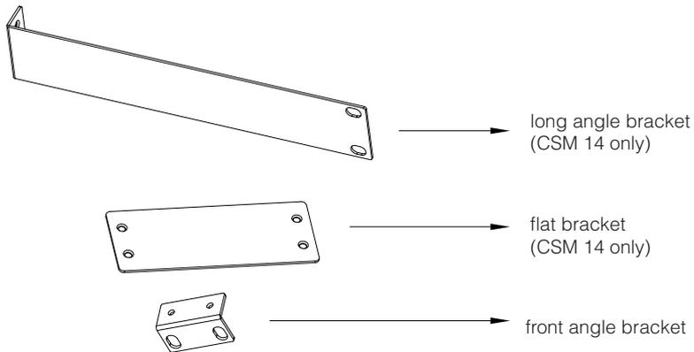
Figure 2.2.3 Rack Mounting Two Half-rack Mixers
