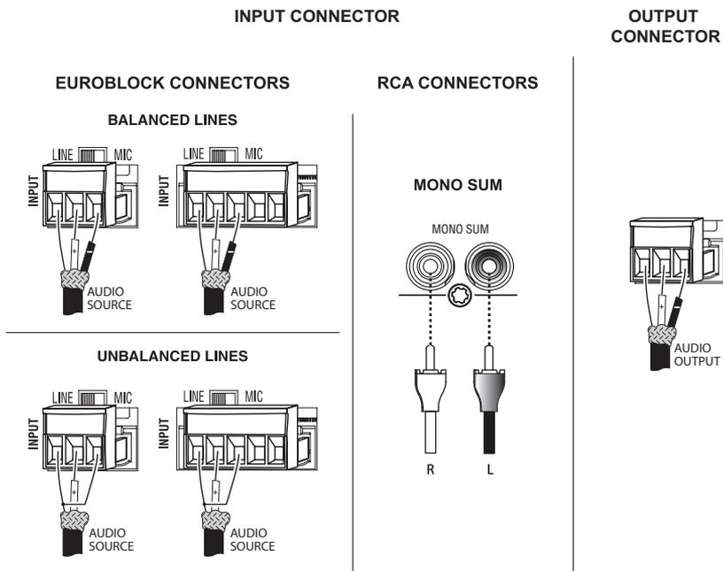
**Note:** Two RCA connectors are provided for summing left and right channels from a stereo source. Do not use both Euroblock and RCA connectors concurrently for any single input channel.
