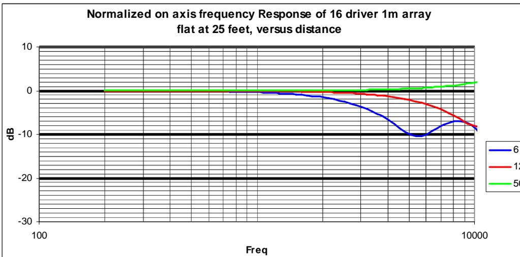
Figure 5. The simulated on and off axis behavior of a finite straight line array of 16 elements 1m tall and the response at 6, 12 and 50 feet normalized to flat at 25 feet. The on axis response changes with distance.
