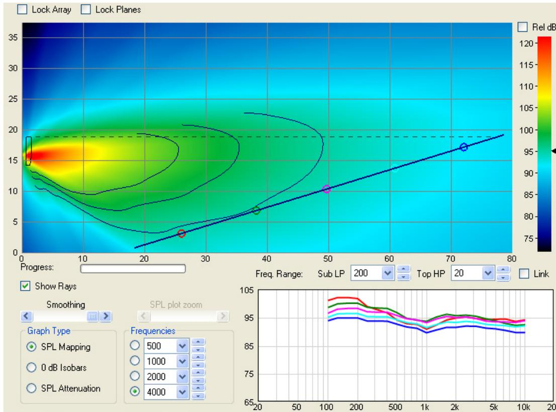
**Figure 15. CBT 70J has tighter pattern control above the speaker and broad downfill capability below. The CBT 70J has excellent front to back evenness of coverage. Note response variation (in lower right corner) from front to back is only 5dB from 500 Hz and above. (From CBT calculator). The frequency response at 5 evenly spaced locations is clearly indicated with color coding.**
