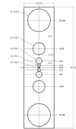
Fig. 15. Driver locations and front panel layout for the example five-way constant-beamwidth loudspeaker system. The system uses two 15" sub woofers, two 8" woofers, two 4" lower midranges, two 2" upper midranges, and a single 1" dome tweeter. The driver spacing ratios are indicated with "x" prefixes. All dimensions in inches.
