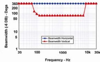
Fig. 17. Beamwidth (-6 dB) versus frequency of the example five-way constant-beamwidth speaker system shown in Fig. 15. Note the extreme uniformity of beamwidth which is about 75° between 125 Hz and 6.3 kHz. At 7.4 kHz and above, the tweeter (assumed to be a point source) is radiating by itself and provides an omnidirectional 180° response. This can be corrected by using a tweeter with an inherent controlled high-frequency coverage.
