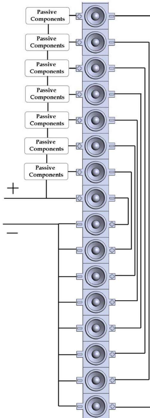
**Figure 9. The passive CBT principle utilizing a ladder of passive components to create a delay line with increments of group delay to mimic the performance of a digital delay derived CBT array. The components chosen for a given arc can be changed to provide new arc if the pattern were required to change.**
