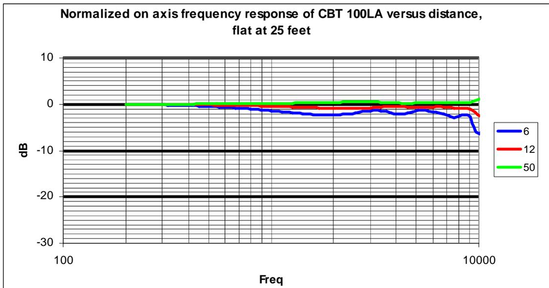
Figure 11. CBT 100LA response variation with distance is very consistent with distance as compared to straight array in figure 5.
