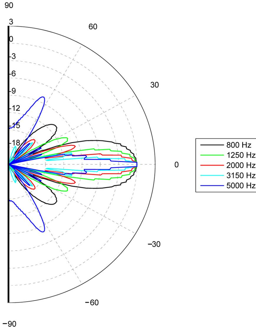
**Figure 6. The measured vertical polar patterns from a popular straight line array of 1m in height with 12 discrete drivers. Side lobes can be seen as low as 800 Hz. The pattern continuously narrows with frequency and has clear lobes outside the main lobe.**
