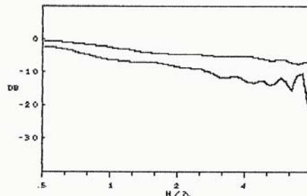
**Figure 3. From Augspurger and Brawley<sup>4</sup> showing that relatively even coverage off axis can be obtained with delay and that with the addition of Bessel shading very smooth off axis behavior can be obtained.**
