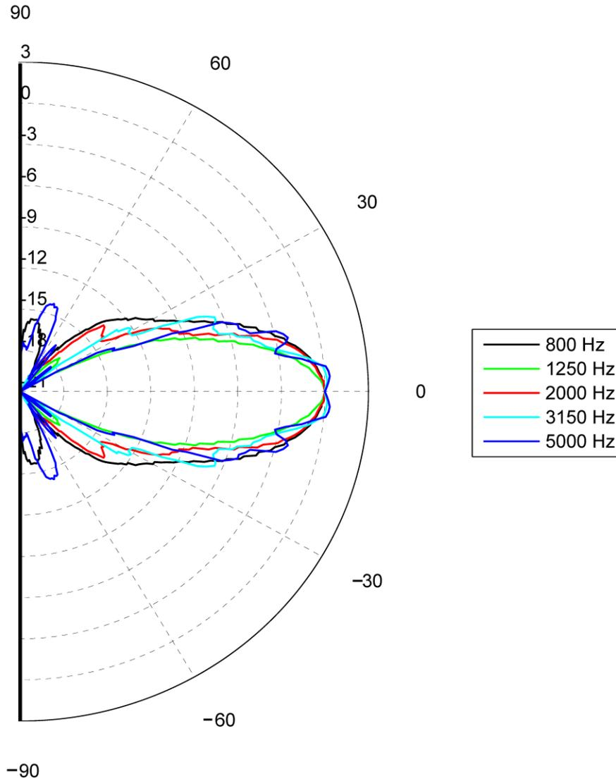
**Figure 12. The measured polar patterns from a CBT 100 LA 1m in height. Compared with the straight array in figure 6, the pattern is very uniform with frequency with virtually no side lobes.**
