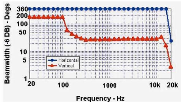
Fig. 57. Farfield above-ground-plane beamwidth (-6 dB) versus frequency for an Legendre-shaded 50-point 1.25m-high 45° curved-line source located on a ground plane (Fig. 56). Horizontal: blue circles. Vertical: red triangles. Note the extreme uniformity of vertical beamwidth with frequency.
