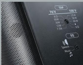
**USER VARIABLE VOICING** The Music/Speech switch (on all CBT models) allows quick and easy adjustment of the response. Music mode provides a flat, balanced frequency response, while Speech mode adds a mid-range presence peak for enhanced speech intelligibility. So, regardless the application, the CBT Series can be tailored to suit the need.
