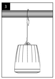
3. With speaker supported, snap main support hook hanger onto the center hole in the top bracket of the speaker. Adjust to proper height by pulling cable through either end of Gripple.
