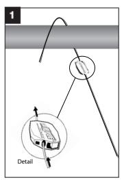
1. Thread Gripple onto cable (see inset detail). Pass over ceiling anchor point (as shown) or through other secure anchor point of the building structure. Installer is responsible for ensuring that anchor point is secure to building structure.
