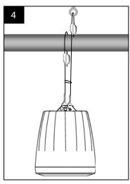
4. Snap secondary support safety cable hook hanger onto one of the side holes in the top bracket of the speaker, and attach the top to a different ceiling support point of the building structur e, per Steps 1 & 2. After height adjustment is final, trim any unneeded extra cable tail wires with trimmer suitable for 2 mm (0.077 in) diameter stranded aircraft-type cable.
