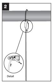
2. Pass tail end of cable through the other channel of the Gripple (see inset detail).
