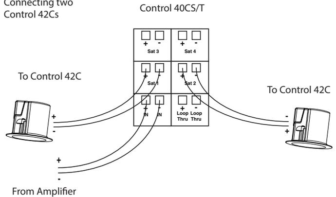
If using four Control 42C satellites, connect each loudspeaker to a single output connector as shown in the diagram below, one Control 42C to "Sat 1", the second Control 42C to "Sat 2", the third Control 42C to "Sat 3", the fourth Control 42C to "Sat 4."
