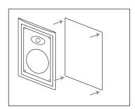
Place the frame assembly in the wall.
