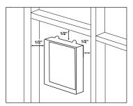
**Note:** Always allow at least one-half inch between a wall stud and the speaker cutout or the locking tabs will not be able to swivel into place.
