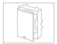
Remove the grille from the speaker frame by pulling on the paper tab. If the tab is missing, to avoid scratching the grille or baffle you may unfold a paper clip, insert the straight end through one of the holes in the grille, and gently pull up.
