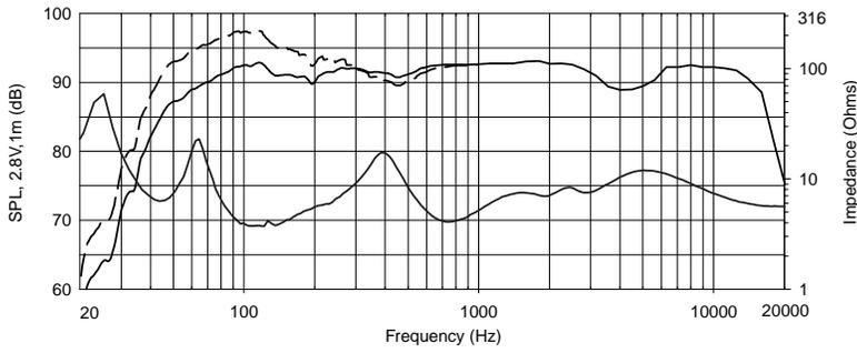
Frequency Response, on axis in half-space ( $2\pi$ , dotted line) and full space ( $4\pi$ , solid line) at thru ( $8\Omega$ ) setting, Input Impedance.
