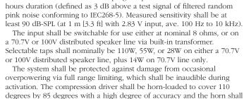
transducer, 25 mm (1 in) compression driver, and frequency dividing network. The low frequency driver's voice coil shall be 50 mm (2 in) in
