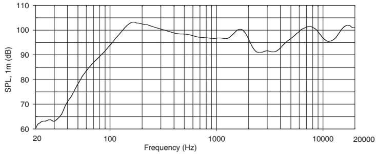
Frequency Response, on axis in half-space, 70V input to 25W tap
