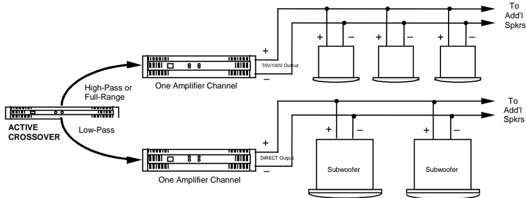
*Note: JBL MPC-T amplifiers have the ability to simultaneously drive a 70V/100V line from one channel and low impedance speakers on the other channel, such as shown in diagram.*
