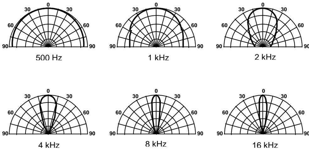
*Based on 165 mm (6.5 in) radiating diameter*
