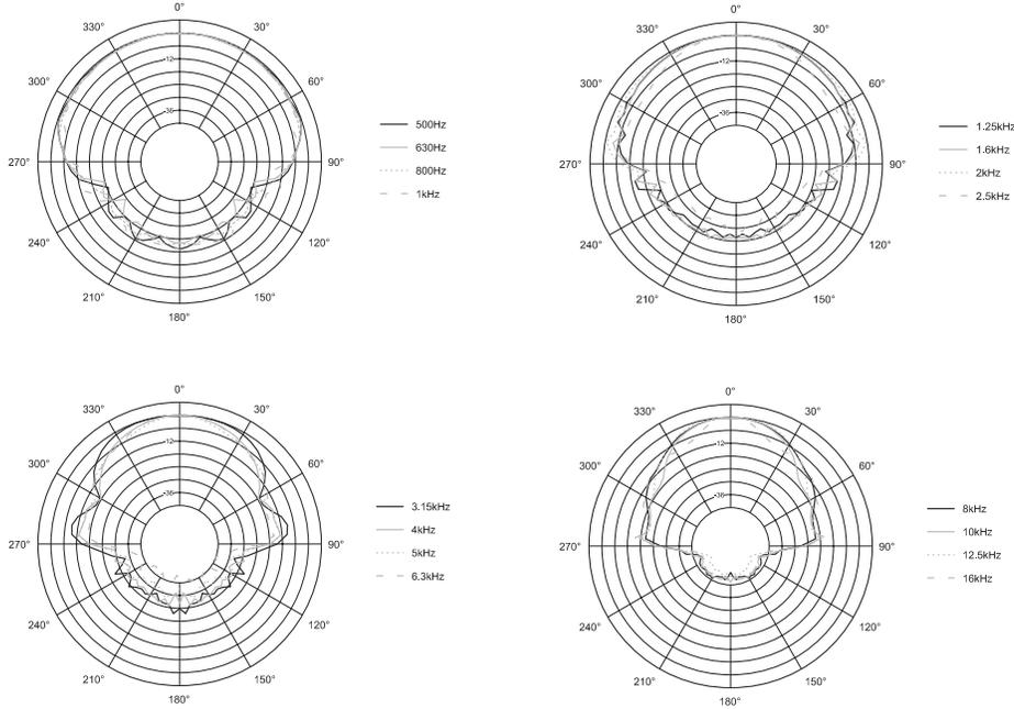
**Single Speaker Coverage** – The coverage area of a single speaker depends on the distance of the speaker from the listener, which depends upon the ceiling height and the listening height (seated vs. standing). The following chart assumes a 4 ft (1.2 m) listening plane and averages coverage over the 500 Hz to 8 kHz range:
