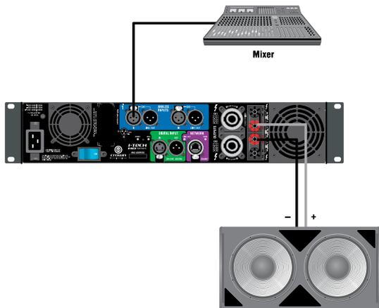
1. Wire the speaker across the red binding post of each channel. Do not use the black binding posts when operating in Bridge-Mono mode.
