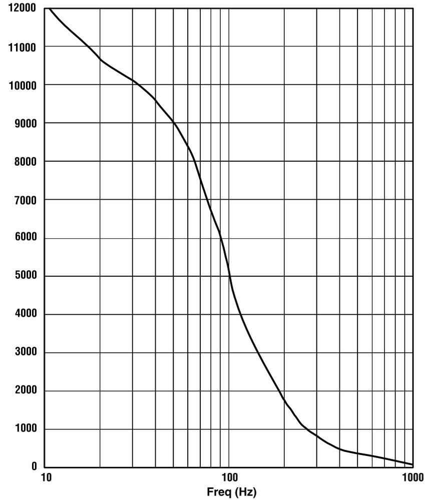
Typical Damping Factor vs. Frequency
