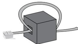
When using network connections, pass the CAT 5 cable five times through a ferrite core, available from Crown Audio Inc. This is to ensure compliance with emission regulations.
