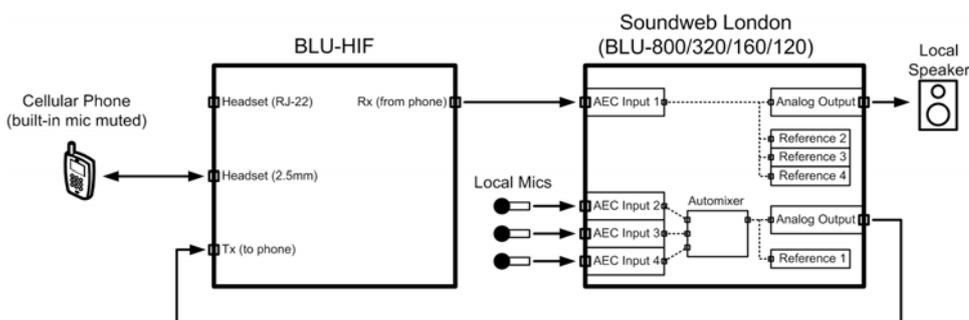
Figure 3: Wiring Diagram – BLU-HIF Telephone Headset Jacks
