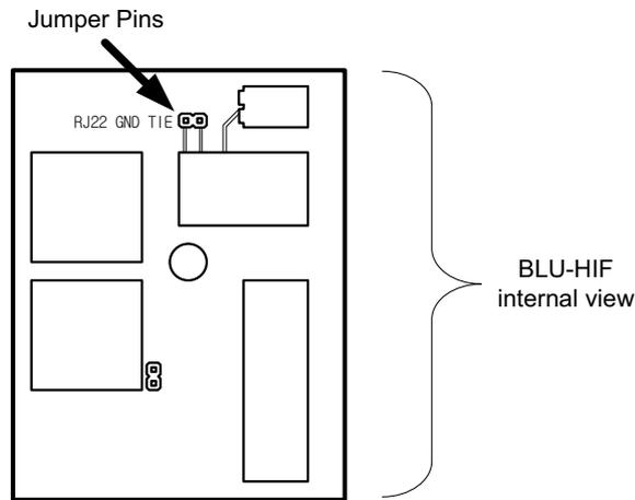
Figure 5: Setting the Internal Jumper
