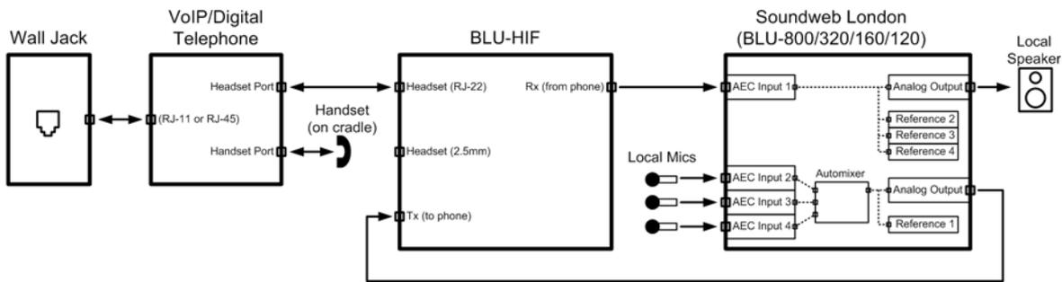
Figure 2: Using the BLU-HIF with a Phone Equipped with a 2.5mm TRS Jack
