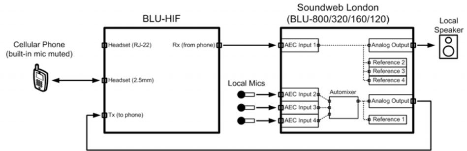
Figure 3: Wiring Diagram – BLU-HIF Headset Jacks
