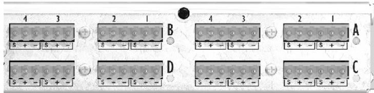
These connectors provide the balanced connections for the I/O card fitted in the four card slots in a Soundweb London device. A green LED next to the slot assignment letter A, B, C or D indicates that an Input card is fitted and an amber LED when an output card is fitted. The analogue connections are balanced, on Phoenix/Combicon connectors. Digital input cards are indicated with a blue LED and digital outputs cards with a red LED.
