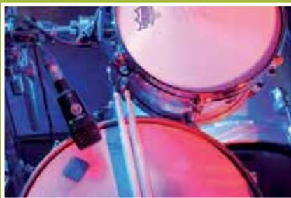
Place the microphone so that it points away from the hi-hat in order to minimize leakage from the hi-hat into the snare drum channel.
