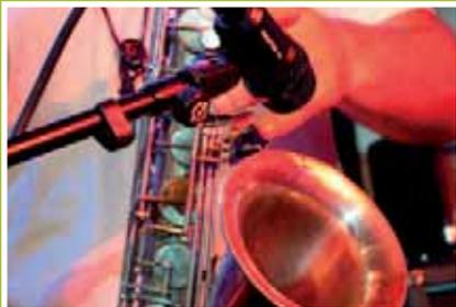
Always place the microphone as close to the sound source as possible! This minimizes the amount of unwanted sound (e.g. from other instruments) picked up by the microphone.
