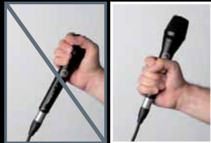
Microphones with cardioid or hypercardioid polar pattern are the most frequently used mics on stage. It is very important to hold the microphone correctly. Take care not to cover the sound inlet basket with your hand, as this will have an unfavourable effect on the polar pattern, while also increasing feedback risk quite considerably.
