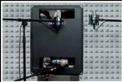
Miking with three microphones will ensure an eminently spatial effect. Point one microphone at the low-frequency driver from a distance of about 8 inches. Place two other microphones at a large aperture angle so that they are directed at the high-frequency driver from a distance of about 8 inches.
