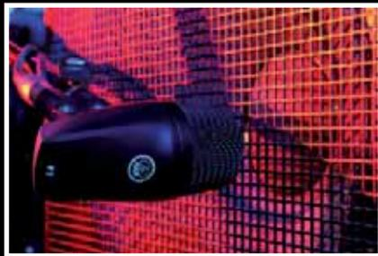
E-bass or guitar are frequently picked up quite "dry" via a DI Box. By contrast, using a microphone will also reproduce the characteristic sound features of amplifier, loudspeaker box and space, thus delivering a more lively sound. Blending the two signals will frequently ensure optimum results.
