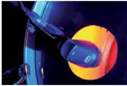
The engineers at the AKG acoustic research laboratory tested the P 2 with many different kick drums. To get the best possible sound, they recommend a 3 dB boost at 70 Hz and a 3 dB cut at 700 Hz on the EQ (e.g., on the mixer).
