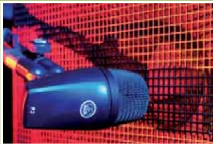
To mic up an amp, place the microphone as close as possible to the speaker. As you move the microphone toward the center of the diaphragm, the sound will become brighter.
