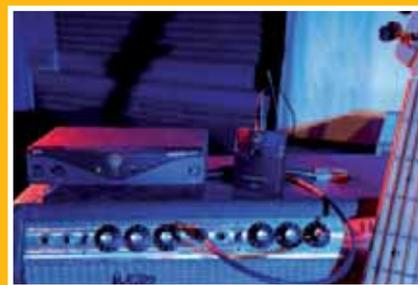
Radio waves are similar to light. Therefore, always place the receiver clear of any potential visual obstructions and wear the bodypack on the guitar strap or on the outside of your clothes so it can always “see” the receiver.
