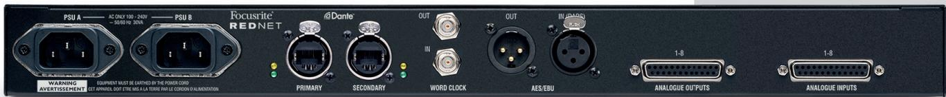
The analogue inputs and outputs are electronically-balanced and provided on 25-way female DB25 connectors wired to the AES59 standard, with internal signals fully-balanced throughout. The inputs and outputs may be configured remotely for either +18dBu or +24dBu operation.
