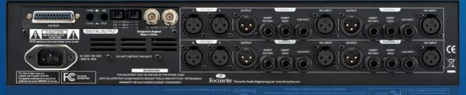
Rear image features the A-D converter card - not fitted as standard
